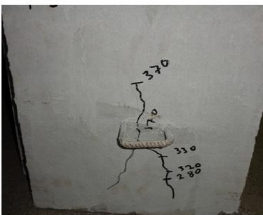
(b) TS Specimen Failure
